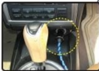
Insert The Plug Of The Electric Car Jack Into The Car Lighter
